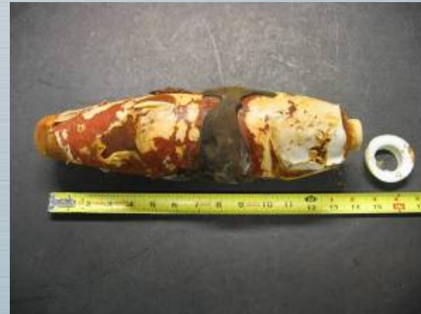
120mm Mortar Following Acid Digestion
