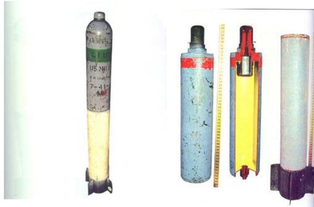
Figure A-2 - The warhead and motor of the 5-inch Rocket
