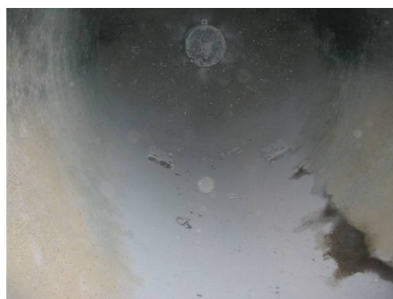
Fig. 3 Inside of DAVINCH detonation chamber after detonation
