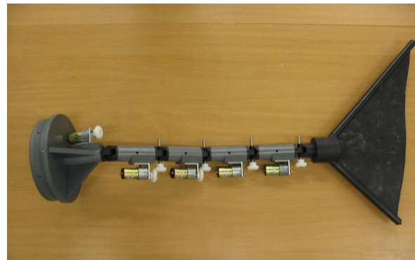
Figure 7: Completed tail assembly
