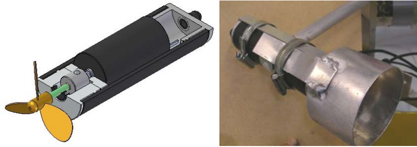
Figure 6. (a) Propulsion modules with (b) associated mechanical fastening system to submarine frame
