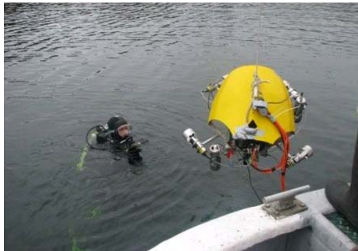
Figure 7 – The Hawthorne being deployed into the open Pacific from a fish boat in western Canada. The racehorse AUV turned workhorse ROV was used for ecological research on mysid crustaceans, which required it to dive repetitively to depths of 20m.
